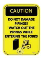
TEFCOLD Refrigeration manufactures its refrigerated cabinets suitable to be lifted using a suitable forklift. Care must be taken to place the forklift forks into appropriate areas underneath the cabinet.
