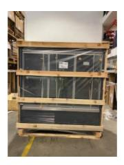
Unscrew retaining screws wood from the wooden pallet with using proper instrument
