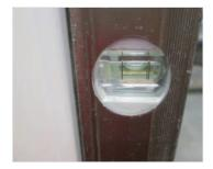
The spirit level is located vertically as seen above pictures. Bubble of spirit level must be positioned in the middle if rear, front and middle feet are levelled correctly.
