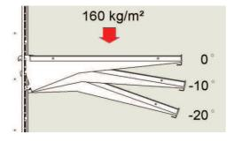
Do not exceed the loading capacity on pans and shelves. (160 kg / m<sup>2</sup>)
