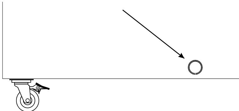
Place a container under the valve to collect melted water.
